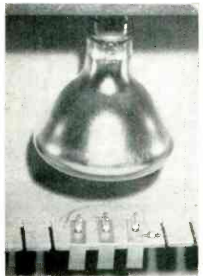
Using infrared heat to solder hermetic-seal terminals to thin metal cover
