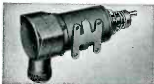
#4440 a continuous service solenoid, 24v, D.C.—3.6 amp. (starting) .42 amp. (holding)—stroke 3/8" weight 16 oz.
