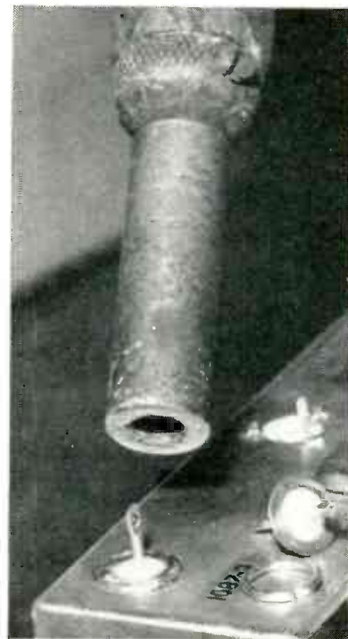
Modified soldering-iron used for soldering feed-through terminals to chassis
