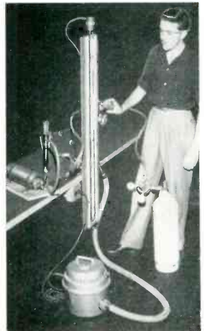
Setup for detecting pinhole leaks in body housing of military electronic gear. Plumber's torch is on bench at left, next to dummy cover panel, and Freon gas tank is on floor at right
