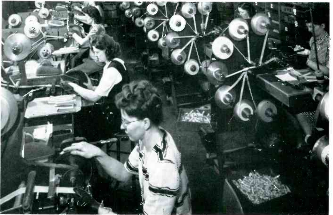
ROLLING ELECTROLYTIC CAPACITORS with "Scotch" Electrical Tape No. 42 at The Magnavox Company, Fort Wayne, Indiana.
