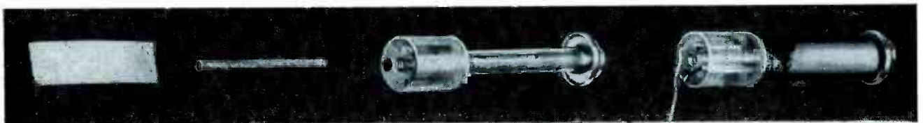
FIG. 2—Straight tubular core magnetor requires considerable shielding to eliminate spurious signals from ambient fields. Permalloy sheet at left is rolled into cylinder and placed in 2-in-long methacrylate pool
