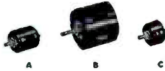
MODELS A, B, & C HELIPOTS A—10 turns, 46" coil, 1-13/16" dia., 5 watts—resistances from 10 to 300,000 ohms. B—15 turns, 140" coil, 3-5/16" dia., 10 watts—resistances from 50 to 500,000 ohms. C—3 turns, 13-1/2" coil, 1-13/16" dia., 3 watts—resistances from 5 to 50,000 ohms.
