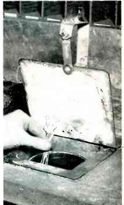
Fire in rosin pot is snuffed out automatically by lid when heat of flame melts solder in overhead link serving as catch in Camden plant of RCA Victor
