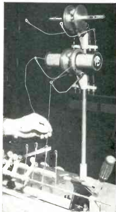
Tips of casting rods serve as guides for wire on coil-winding machine
