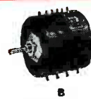
MULTITAPPED MODEL B HELIPOT AND 6-GANGED TAPPED MODEL F This Model B Helipot contains 40 taps, placed as required at specified points on coil. The Six-Gang Model F Potentiometer contains 19 additional taps on the middle two sections. Such taps permit use of padding resistors to create desired non-linear potentiometer functions, with advantage of flexibility, in that curves can be altered as required.
