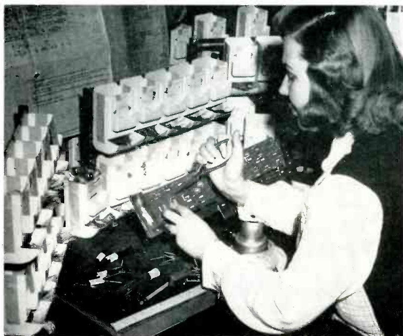
Safety-match holders costing only 11 cents each hang on horizontal bars of racks
