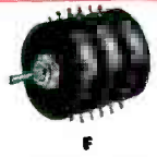
MULTITAPPED MODEL B HELIPOT AND 6-GANGED TAPPED MODEL F This Model B Helipot contains 40 taps, placed as required at specified points on coil. The Six-Gang Model F Potentiometer contains 19 additional taps on the middle two sections. Such taps permit use of padding resistors to create desired non-linear potentiometer functions, with advantage of flexibility, in that curves can be altered as required.
