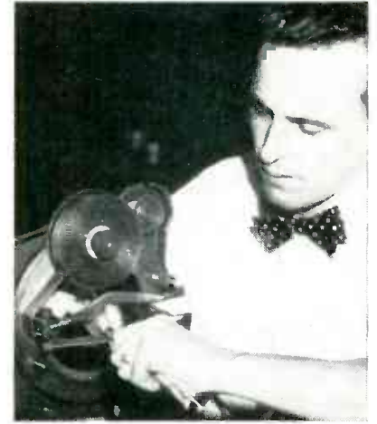
Winding Scotch electrical tape on formed cable harness with modified Segur taping machine
