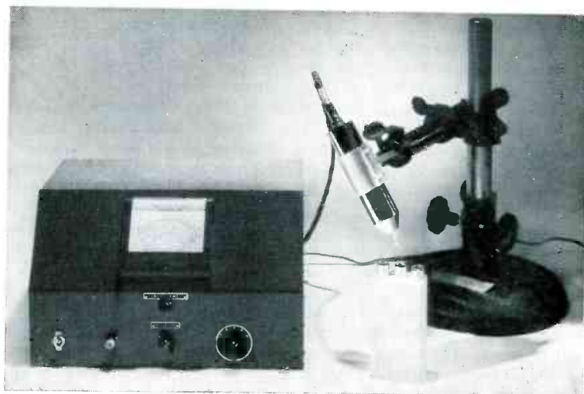
Complete system of the vibrating-plate viscometer
