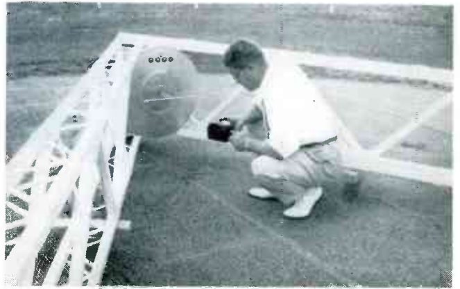
FIG. 2—Checking the operating frequency of a target transmitter. Unit derives its power from wet-cell batteries
