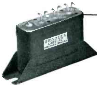
SELENIUM RECTIFIER SR 114 USED AS PRECISION LIMITER
