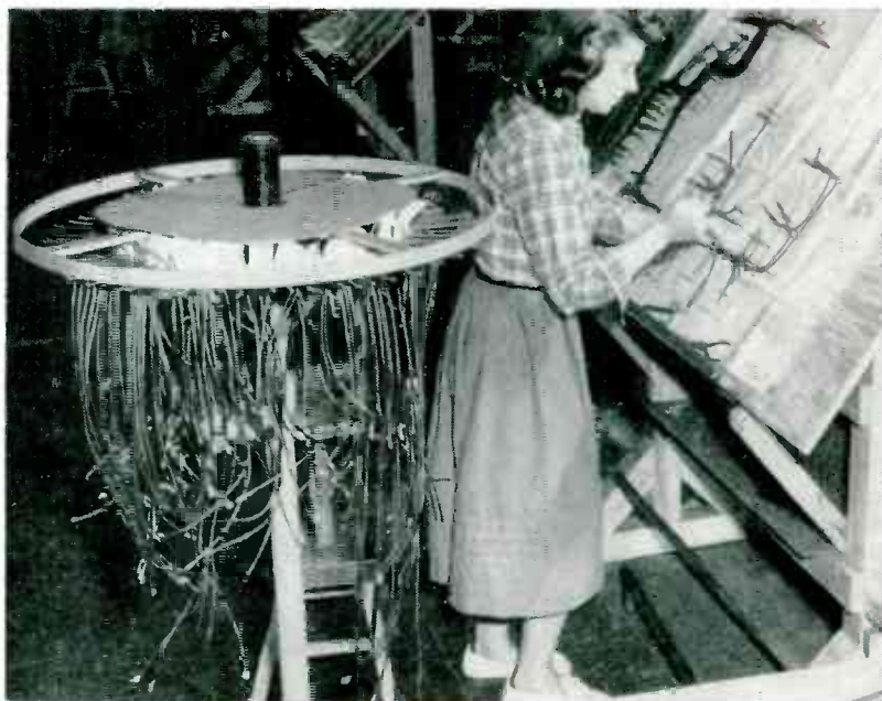
Holder for precut lengths of wire used in forming cable harness at GE plant. Circular wood rim is convenient for turning holder. Spool of lacing cord is on top
