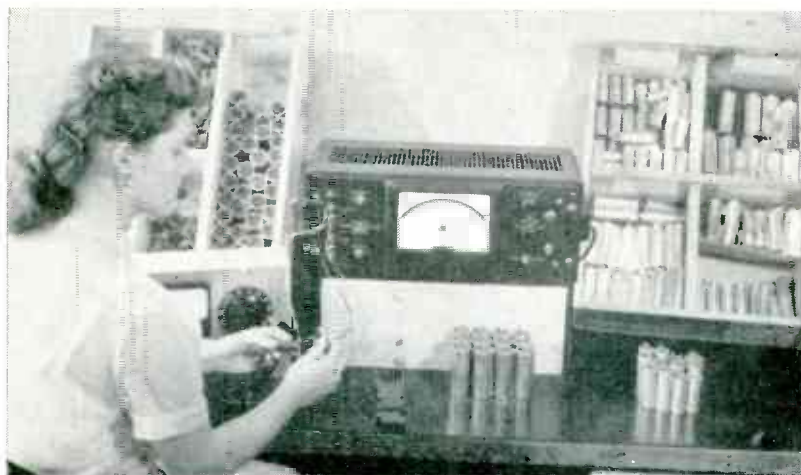
Setup for checking loss of electrolytics as fast as they can be placed across a pair of test terminals
