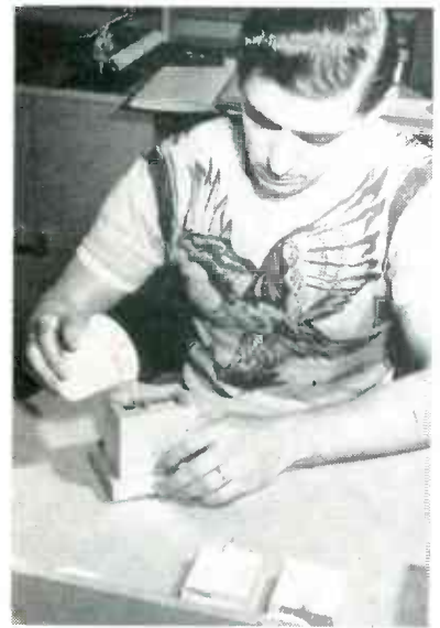
Pouring resin from disposable paper cup into mold containing Hamilton Standard's electronic subassembly for controlling flow of fuel to aircraft gas-turbine engines. Potted units, after removal from mold, are shown in foreground
