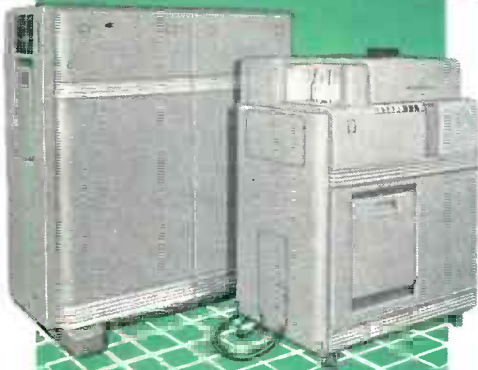
The large cabinet is the all-electronic unit; the smaller is the electrical card reading and punching unit.
